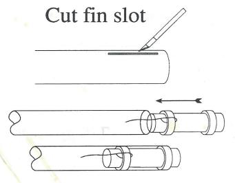
8) Epoxy the fins into the fin slots in the body tube. Make sure they are straight with the body tube. For maximum strength give the fins a good fillet coat of epoxy.
