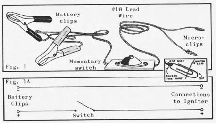
With such a system you must take care never to connect to the battery until after the clips have been connected to the igniter leads.
