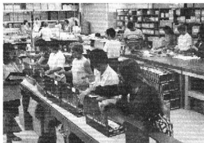
This conveyORIZED setup in one section of the kit packing department has more than doubled kit production.
