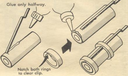
Apply glue around end of engine compartment. Place centering ring so that it is on this glue and flush with the end of engine compartment, and engine block. Place a line of glue, and the other centering ring about an inch from the other end.
