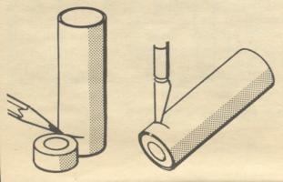
Cut slit on the pencil mark, and insert engine clip. Apply glue in a straight line so that the engine clip will drop into it. Press firmly, and wrap a piece of tape around the assembly, until the glue is hard.
