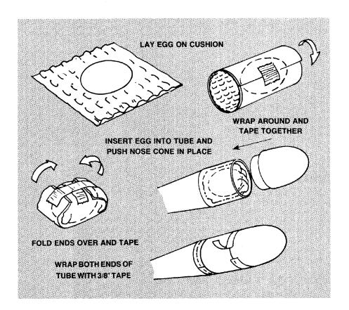
IMPORTANT NOTE: This model may be flown with or without an egg payload. In either case, the egg tube must be firmly taped to the nose and tail cone. Otherwise, these parts might separate when the parachute is deployed, and they could be lost. Careful attention must also be paid to engine selection. Page 6 lists a range of engines that may be used to power this rocket when it is flown without an egg payload. When launching with an egg, use only an Estes C5-3 engine.
