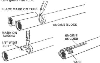
☐ 3 The engine holder is attached to the engine tube with one of its hooked ends against the engine block. To locate, hold the casing against the outside of the engine tube with the mark on the casing even with the end of the tube. Place a mark on the tube even with the top of the casing. Cut a 1/8" wide slit in the tube on the pencil mark. Insert one end of the engine holder into slit. Align holder with tube and temporarily secure with a piece of masking tape around bottom of tube.
