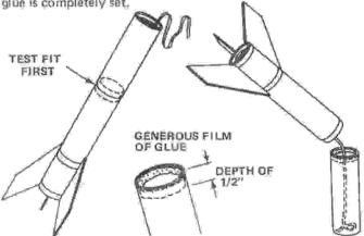
12 After the glue has dried on the main rocket assembly, attach the remaining body tube. Test fit the tube on top the assembly. If necessary, lightly sand the inside edge of the tube
