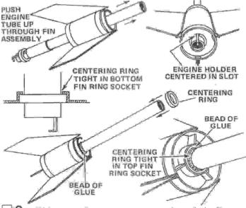
9 Stide the engine tube assembly up through the fin assembly as shown. Note that the engine holder must be centered
