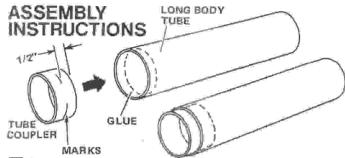
1 Mark the tube coupler [part L] in the middle (1/2" from one end). Put 3 or 4 marks around coupler so it can be positioned straight in the body tube. Run a bead of glue around the inside of one end of one 9" long body tube (part K). Push the coupler into the tube until the marks on the coupler line up with the end of the tube. Wipe away excess glue and set aside to dry.
