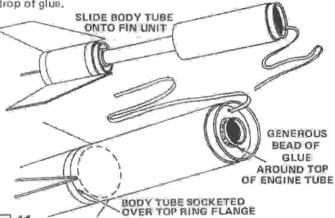
Slide the body tube assembly onto the fin unit. The bottom of the body tube should be socketed over the upper section of the fin ring and the engine tube should extend through the die-cut ring at the top of the body. Make sure the whole unit is pushed tightly together, then apply a generous bead of glue to the engine tube where it protrudes through the die-cut ring. Set the assembly aside and do not disturb until glue is completely set.
