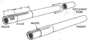
Place a mark on the engine tube 1" from the end. Smear a film of glue around the tube above this mark for a distance of 2". Make sure you have glue all around the upper portion of the engine holder. Slide the retainer tube onto the opposite end of the engine tube. Push the retainer down until it reaches the 1" mark. Wipe away excess glue.
