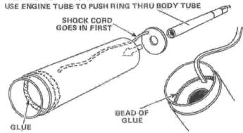
Locate the body tube and coupler which you glued together in step 1. Apply a bead of glue around the inside of the body tube at the base of the coupler. Insert the die-cut ring into the opposite end of the body tube with the shock cord extending through the body first (as shown). Use the engine tube to push the ring through the body tube until the ring is tight against the bottom of the coupler. Apply a second bead of glue around the ring-coupler joint and set aside to dry.
