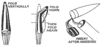
T-12 Loosely fold the parachute. Lay it on top of the wadding, with its shroud lines and shock cord on top of it. Slide the nose cone into place.
