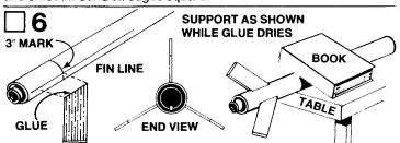
The fins are attached to the body, centered on the fin lines with the front edge of each fin on the 3" mark. Apply a bead of glue to the root edge of one fin. Allow the glue to set for a couple of minutes, then attach the fin to the body. Make sure the fin extends straight from the body. Lay the assembly on a table with the fin pointing up. Lay a book (or similar object) on the front of the body so it won't roll. Allow the glue to dry completely. Attach the remaining fins in the same manner.
