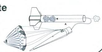
**Install Igniter and Rocket Motor**
