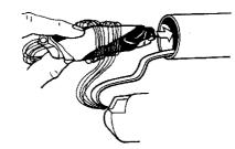
3. Install the nose cone into the forward end of the rocket body. Be certain the fit is neither too loose or too tight. If the nose cone falls out of the rocket body when the model is pointed downward, the fit is too loose. If while pointed downward, the nose cone can't be shaken out of the tube, the fit is too tight. If too loose, wrap tape around shoulder for snug fit. If too tight, lightly sand shoulder slightly for looser fit.
