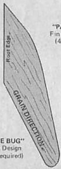
"CLOUDBUSTER 1" Fin Design (4 required)
