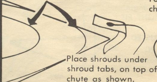
Place shrouds under shroud tabs, on top of chute as shown.
